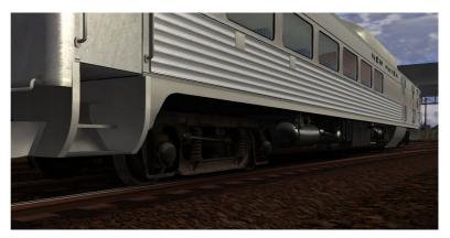
They give the RDC a high power-to-weight ratio of 8.68 horsepower per ton. Each engine drives one axle on its adjacent truck, giving the RDC exceptional acceleration and also allowing it to continue on its journey at reduced speed in case one engine fails.
