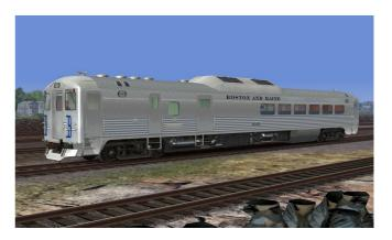
RDC's were offered in four configurations: the RDC-1, with seating for 89 passengers, the RDC-2, with seating for 70 passengers and a small baggage compartment, the RDC-3, which offered space for 48 passengers and had both baggage and mail compartments, and lastly the RDC-4, designed exclusively for mail/express cargo.
