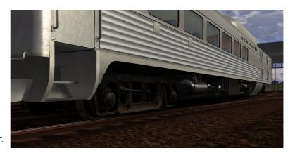
to-weight ratio of 8.68 horsepower per ton. Each engine drives one axle on its adjacent truck, giving the RDC exceptional acceleration and also allowing it to continue on its journey at reduced speed in case one engine fails.
